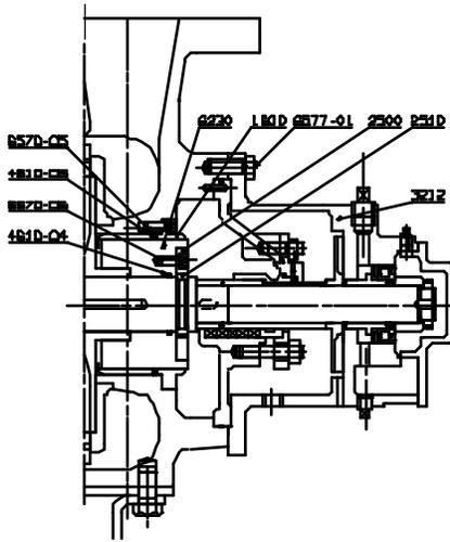
Dismount the line bearing assembly; see section 6.8.3.
