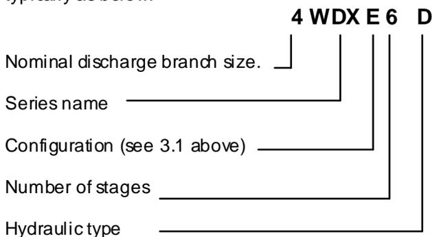
The typical nomenclature above is the general guide to the WDX configuration description. Identify the actual pump size and serial number from the pump nameplate. Check that this agrees with the applicable certification provided.
