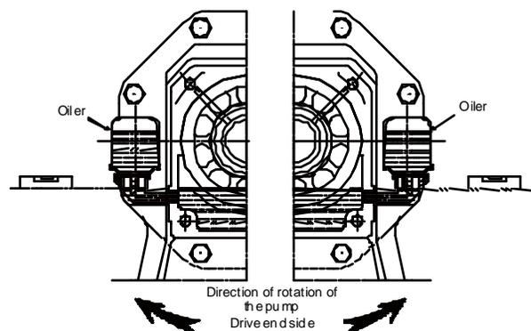
When fitted with a constant level oiler, the bearing housing should be filled only by unscrewing or hinging back the transparent bottle and filling the bottle with oil. Do not fill the bearing housing through the breather hole.
