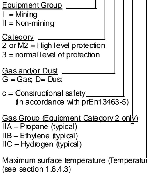
**1.6.4.3 Avoiding excessive surface temperatures**
